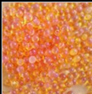
Amber Silica Dehydrating Beads
